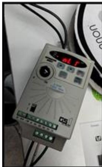
**Fig. 5** Controlador Automation Direct® Serie GS1, 0.5 HP.
